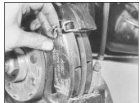
3.8A Disc pad and anti-rattle spring
