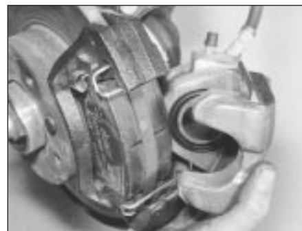
3.4 Removing the caliper unit
