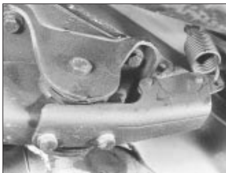
10.4 Pressure regulating valve bracket and tension spring
