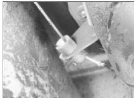
17.3 Handbrake cable guide on fuel tank
